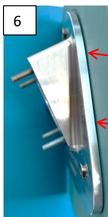
6 There should be a slight interference fit to the body on the screws that are now studs, to keep them from spinning.
